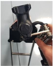
4. Place the handle bars back on along with the bracket and start by hand tightening the four screws to get the threads started. Then tighten the screws in a pattern using the multitool so all screws will be tightened down evenly.
