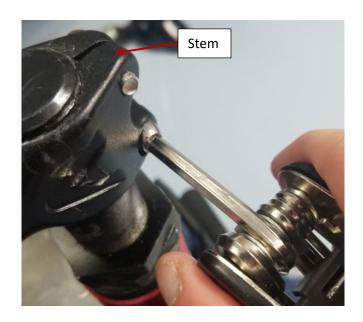
3. Rotate the stem 180 degrees and looking down from the top of the EZ-Ride and line up the stem with the drive wheel. Once both are lined up properly, tighten the stem down switching between the two screws so they are both tightened down evenly.
