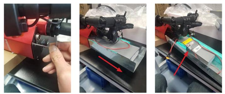
4. Remove the old battery and place new battery on the metal divider with the yellow connector sticking out through the cutout on the divider just like the old battery. Try to use the existing packaging foam to secure the new battery inside the metal divider so the battery does not move.
